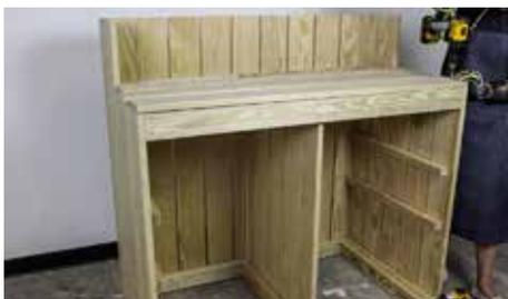
Place a Part (H) on the top surface and secure with 2" screws after ensuring it is flush on all edges.
