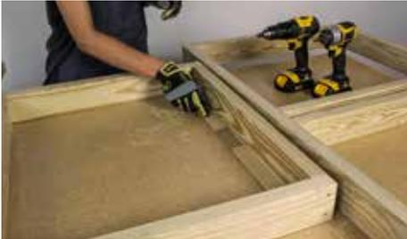
Build a second rectangle frame identical to the first, and then set the first one aside. For the second frame, place  $\frac{1}{4}$ " spacers inside the short ends flat on the table.
