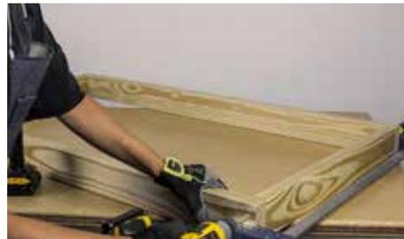
To create the two frames, secure two Parts (D) to two Parts (E) with two  $2 \frac{1}{2}$ " screws per joint to form a 90-degree rectangle. Use bar clamps to help maintain a square joint as needed.
