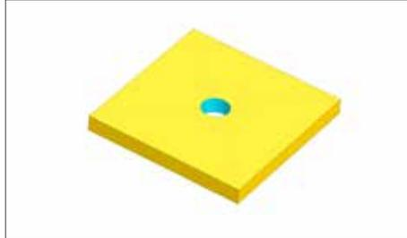
Measure and mark the center of the board by lightly penciling two diagonals from each corner. Clamp the piece to a work table and drill this center-point with a 1 1/4" hole-saw.
