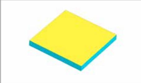
Start by making a square piece out of the 1x8x8' stock by cross-cutting it to the same dimension as its width, or about 7 1/2".
