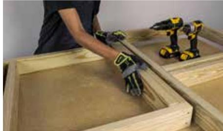
Then, place a Part (E) inside the rectangle's short side on top of the spacers. These will lift the 2x4s a bit so that, when flipped, they are the main feet for the unit.
