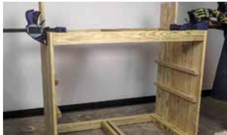
Once the bottom frame is attached to the side walls, place the unit on the ground and secure the top frame so it is flush with the lower part of the side walls. Use clamps as needed, and attach with  $3\frac{1}{2}$ " screws.
