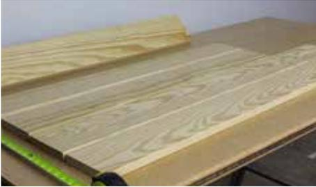
Begin by placing three Parts (A) and two Parts (B) on a flat work surface with  $\frac{1}{4}$ " spacers placed between them. Place the best board faces facedown on the table.
