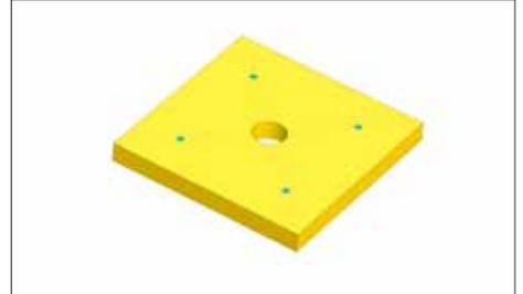
Next, measure and mark four holes on the diagonals using the Diagrams page. Drill with a 3/16" bit.
