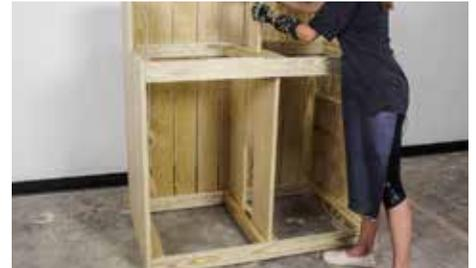
Drop in Parts (F) and (G) in between the center of the frames. Note that Part (G) is ripped so that it will fit easily within the middle frame. It is placed at the back of the middle wall.
