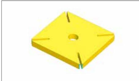
Finally, use a miter saw set to 45° and chop about 1/8" off of each corner to ease the sharp points. You can also use a sander if desired.
