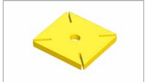
Ease any sharp edges using a radial sander or sanding block with medium grit. Apply preferred finish to the wood. To use, center the piece over the neck of a wine bottle and slide four glasses upside down into the slots. Carry by the wine bottle.
