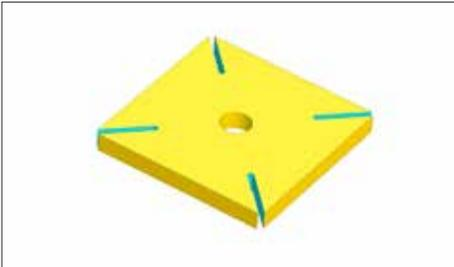
Draw straight lines tangent to the four holes, extending to the corners. Clamp the piece to a work table and insert the jigsaw blade into the 3/16" hole or begin at the corner. Follow the line to make the slots for the glass stems. Do this on all four corners.
