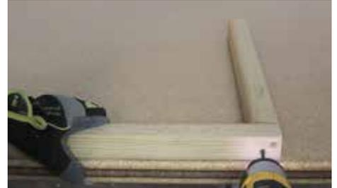
While the leg assemblies are drying, take a Part (B) and (C) and attach them at a 90° angle using a square. Use two 2 1/2" screws at a diagonal as shown.
