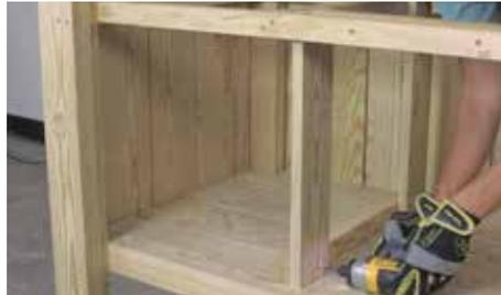
Using the Part (C) you just installed and the (C) directly above, place and attach two Parts (K). Secure the front and back ones to Parts (C) using two 1 5/8" screws.
