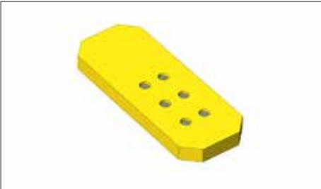
Insert epoxy into the bottom of the holes - about a  $\frac{1}{4}$ " thickness. Then place magnets into the holes, wiping excess glue as you go. The magnets should sit a bit sub-flush of the back surface. Allow epoxy to fully cure.
