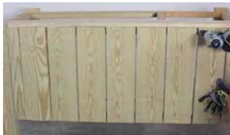
Attach the back slats starting with the two end pieces, Parts (J), and filling in with Parts (I), evenly spacing as you go.
