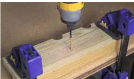
Attach Part (M) to Part (L) so that their bottoms are flush using three 1 5/8" screws. Clamp as needed.
