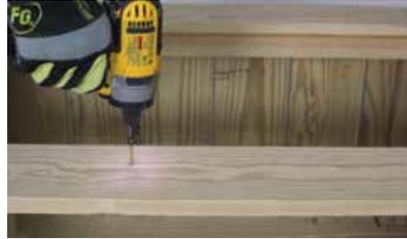
Attach the other Part (N) to the front using five 1 5/8" screws.
