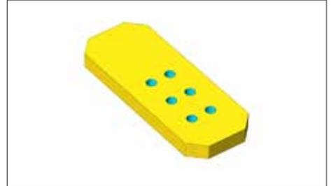
Cut holes using a  $\frac{1}{2}$ " forstner bit to  $\frac{1}{2}$ " depth.
