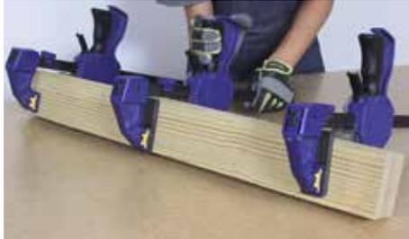
Ensuring all edges are flush, carefully clamp the set of three together using three clamps. Repeat until you have four leg lay-ups and set aside to dry for the indicated amount based on the wood glue of your choice.
