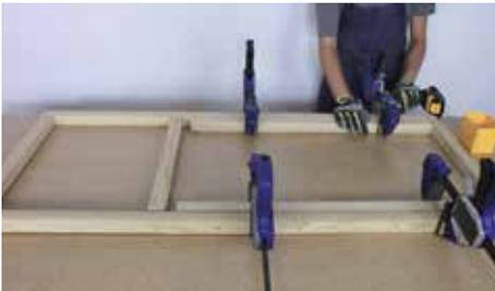
Place two Part (D)s inside the larger cavity in the frame. Space them so they are flush with the right side and 7/8" from the middle (C). Clamp as needed and secure with five 2 1/2" screws, avoiding any existing screws.
