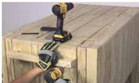
Attach (U) so it is 2 3/4" down from the top of the cooler and centered between the right legs. Use four 3" screws.
