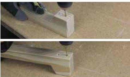
To prep Part (U), pre-drill two sets of holes to back side first and then the front side. Then countersink. Set the holes evenly spaced within the protrusion.
