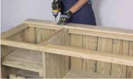
Attach Part (N) to the top surface, evenly spacing between the two back legs. Use five pairs of 1 5/8" screws.
