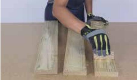
Begin by laying out three Part (A)s with their best faces face down on a work surface. Apply wood glue to their faces and stack the pieces together in a lay-up.
