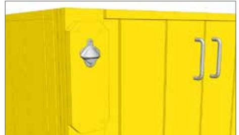
Finish by installing the completed unit onto the left side of the cooler using four  $1 \frac{1}{4}$ " screws at each corner.
