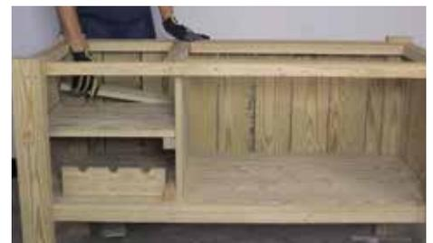
Lay in Parts (K) to the shelf support and evenly space. Attach if desired, or leave loose for more flexibility.
