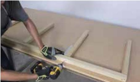
Attach three more Part (C)s in the same manner, where the two inside (C)s are evenly spaced between the two outside ones.
