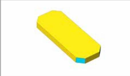
Measure and mark  $\frac{3}{4}$ " from each corner and cut corners with a miter saw set to 45°. Lightly sand the edges of the perimeter.
