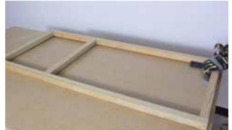
Make a similar frame with two Parts (B) and three Part (C)s, where the middle (C) is placed 14 3/4" from the left (C).
