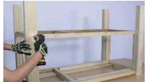
Place and attach the legs at four corners using 3" screws. The frame is inset from the legs the thickness of a 1x6. Next, attach the other frame to the legs 16 3/4" up using four Part (V)s to support it.
