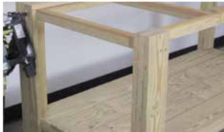
Lay a Part (N) on the top frame. Butt Part (H) up against it, applying pressure to (N). There should be an even gap between the leg, (N), and (H). Use two pairs of 1" nails to attach (H) to the top and bottom frame.
