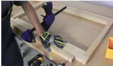
Then, place Part (E) on the outside of (B) so that it is centered. Attach with six 2 1/2" screws, careful not to interfere with existing screws. Put two Part (G)s underneath the second frame.
