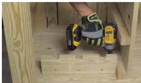
Butt up the assembly to Part (C) on the middle wall and place it 2 3/4" back from the front edge. Secure Part (L) to (G) with three 2" screws. This completes the wine rack.
