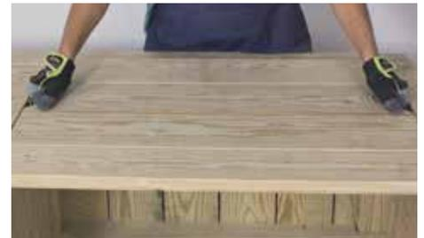
Lay in the lid. It rests in the protruding Parts (D) from the top frame.
