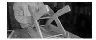
06 Install lock dowels (F) through the pivot dowel (D). Place a piece of folded paper between the legs on either side to leave enough space for easy movement during opening and closing, then drill ¼" holes through the pivot dowel. Coat the lock dowels with glue, insert them into the ¼" holes and pin them in place with finish nails.
