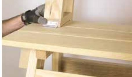
Place the backrest assembly on top of the bench with Part (K) face down. It should be centered and placed at the line you made in the previous step. Ensure that Part (L) has some clearance at the back of the bench.
