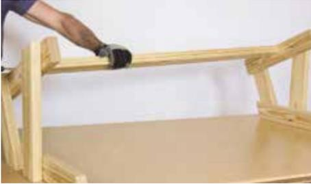
Space two bench leg assemblies apart the length of Part (E), and place Part (E) centered between Parts (A) and Part (D). Clamp Part (E) to Parts (B) so that it is 8 1/4" from the bottom edge of Part (B). Use two 2 1/2" screws per side.
