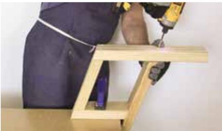
Secure Part (I) to Part (L). Ensure the spacing is the same between Parts (L) and (J) on both sides.
