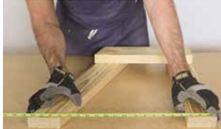
Secure Part (A) to Part (C) with just one screw. Pivot Part (C) until the distance between Part (B) and Part (C) is 20 1/2" .
