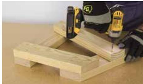
Secure the other end after checking flush.
