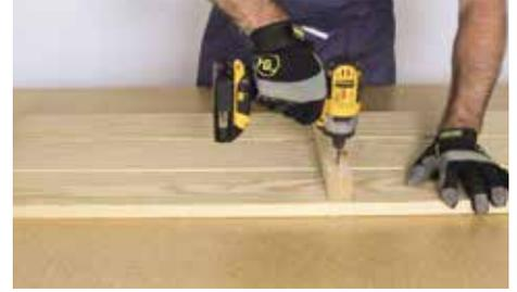
Next, space three Parts (H) on the work surface with their best face down and 1/4" spacers in between them. Clamp the boards together, ensuring edges are flush. Secure one Part (G) centered within the Parts (H) with 2" screws.
