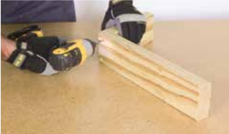
Attach Part (I) to Part (J) using two 2 1/2" screws. Ensure their edges are flush.
