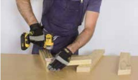
Begin by attaching Part (A) to Part (B), ensuring the top and sides are flush, with two 2 1/2" screws diagonally placed.
