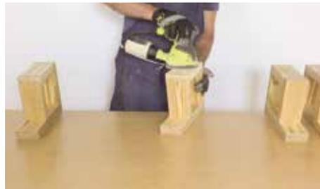
After you've made four arm assemblies, sand all the Parts (I) faces with coarse/medium grit sandpaper with a radial sander or sanding block.
