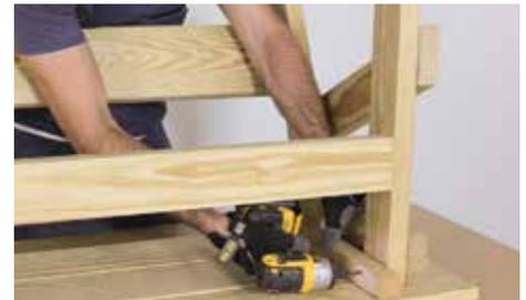
Secure Part (G) to Part (B) and Part (C) on either end with one 2" screw, avoiding the adjacent screws on top of Part (G). Repeat on the other end.
