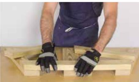
Take the new leg and place it flush with the completed leg to find placement for Part (D).
