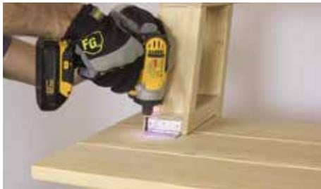
Then you can secure all screw holes in the hinges. Repeat the previous steps on the second bench seat to have two benches.
