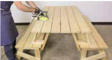
Ease any sharp edges using a radial sander or sanding block with medium grit. Apply preferred finish to the wood.
