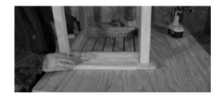
12 Mark locations for "L" bracket placement and drill 1/8" pilot holes ¼" deep in the corresponding holes. Drive screws, making sure the leg/apron assembly draws in tight and remains centered.
