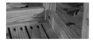
13 Mark center location on the bottoms of all four legs and drill a 1/16" pilot hole about ¼" deep. Hammer in nylon glides, which will prevent the legs from wicking up moisture from the ground or deck.
