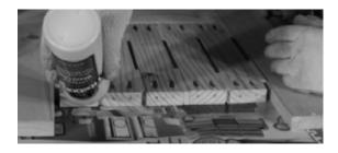
**08** Clamp the assembly together, making sure all edges and faces are flush. Allow to dry.
