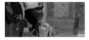
10 Glue and screw apron pieces (E) to the legs (D), keeping top edge of aprons flush with top ends of legs. You can keep the aprons flush with the inside or outside face of the legs if you wish, but in this example, we used ¼" spacers to set them back from the inside face.
