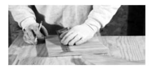
**03** Attach stretchers (C) to the edges of the legs with glue and 1 1/4" screws. Keep the bottom edges flush.
