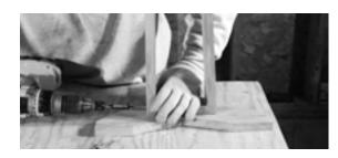
**04** When both stretchers are attached to one side, attach the other foot/leg assembly in the same manner.
