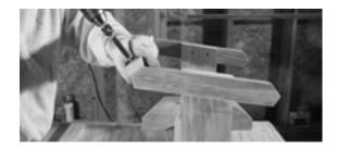
**08** Lay out the rest of your slats, mating the beveled slat edges with each other and filling the middle with unbeveled slats. Put 1/4" spacers between each slat. Attach with glue and 2" screws.
