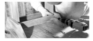
**05** Mark the center points along the top edges of the legs and rails (D), line up those marks and attach the rails to the legs keeping top edges flush.
